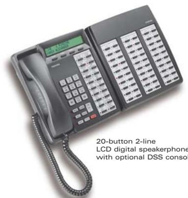
20-button 2-line LCD digital speakerphone with optional DSS console
